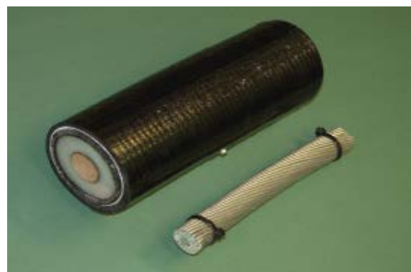
Fig 2. Underground and overhead cable (Georgia Transmission Corp)
