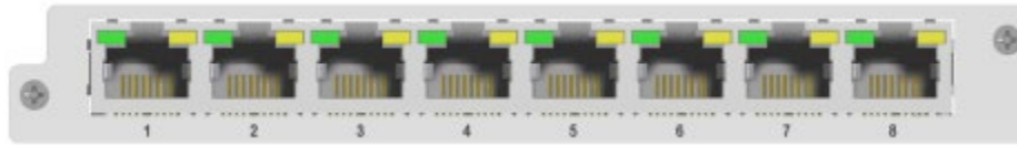
Figure 5-1 8-Channle Camera Input card with RJ45 interface
